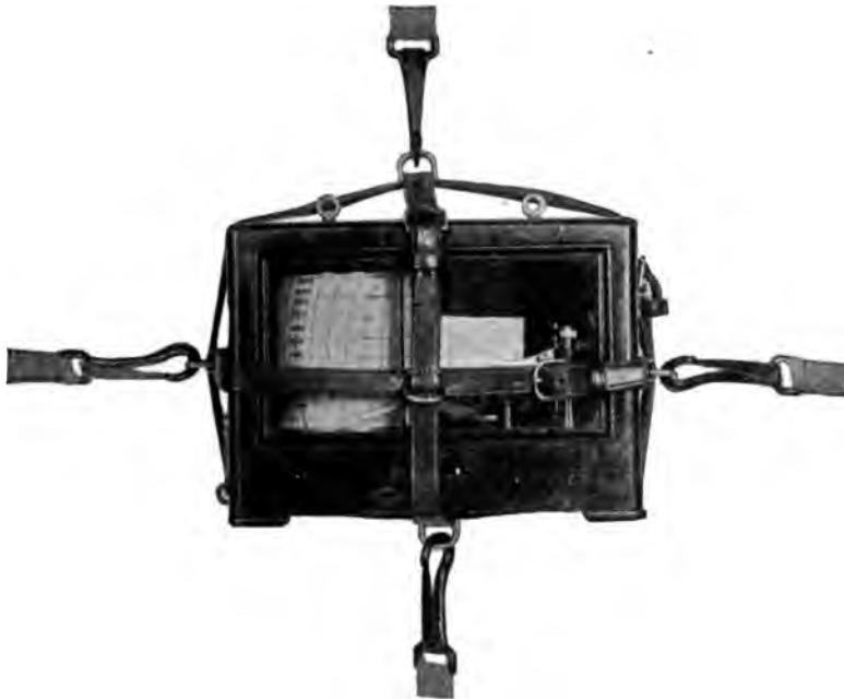
Fig. 35. Barograph Mounted so as to Prevent Vibration
